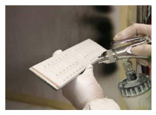
Once the part receives its coating, proper handling is required to prevent issues with the finish. Improper handling will result in contaminants falling on the wet paint, damaging the finish and increasing the likelihood of adhesion problems. In many commercial settings, parts move through a paint booth on a hanging conveyor thereby avoiding manual handling of the wet parts until after curing in the ovens.
