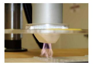
by the blowing of atmospheric air past two high voltage power electrodes. This blowing is often referred to as corona treatment.
